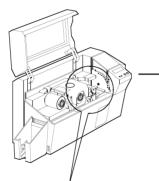
2. Open Printer cover and remove the yellow reminder tape from the location for the Cleaning Cartridge.
